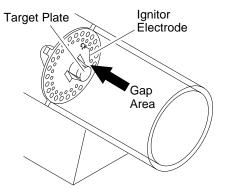
Figure 19 - Clearance between Ignitor Electrode and Target Plate
